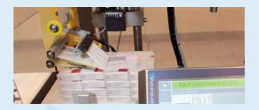
The AR-BASIC AP has a VideoJet DataFlex® 6320 printhead, offering a wide and flexible range of printing in packages as necessary. Once the label has been printed and applied, its information and the legibility are verified.
